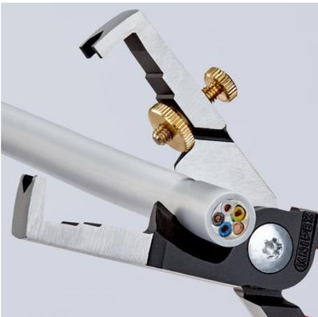
Induction-hardened shear blade with precisely ground cutting edges for crush-free cutting of copper and aluminium Lock nut prevents any unintentional adjustment cables of up to Ø 15 mm (5 x 2.5 mm<sup>2</sup>)
