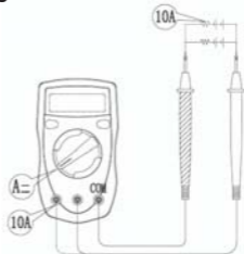
Fig 2. DC Current Measurement
