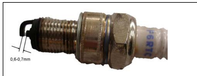
Checking the ignition spark Figure 13: Electrode gap
