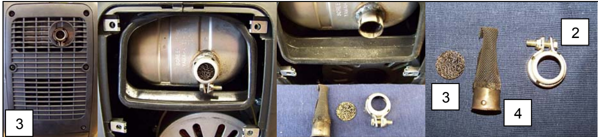
Figure 14: Cleaning the spark catcher
