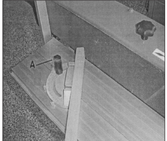
Fig. 7. The scale can be selected and positioned from 45° to 90° at the desired degree by means of adjusting knob A.
