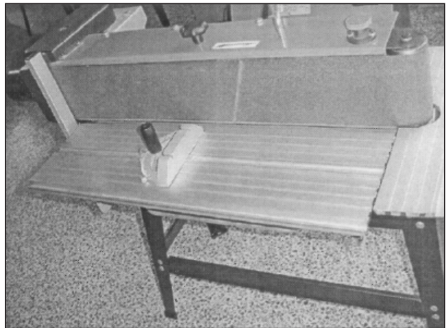
Fig. 2. Adjust the sanding belt to vertical position.
