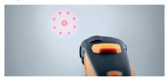
A red laser automatically marks the measurement spot of the infrared thermometer testo 805i. This lets you see exactly what you are measuring – and what not. By the way: you also see this mark in the report you create with the testo Smart Probes App.
