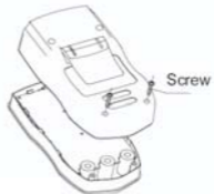
Fig 5. Replacing the Battery Replace the fuse
