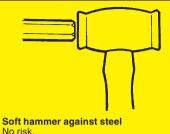
Hammer does not chip. The workpiece keeps its
